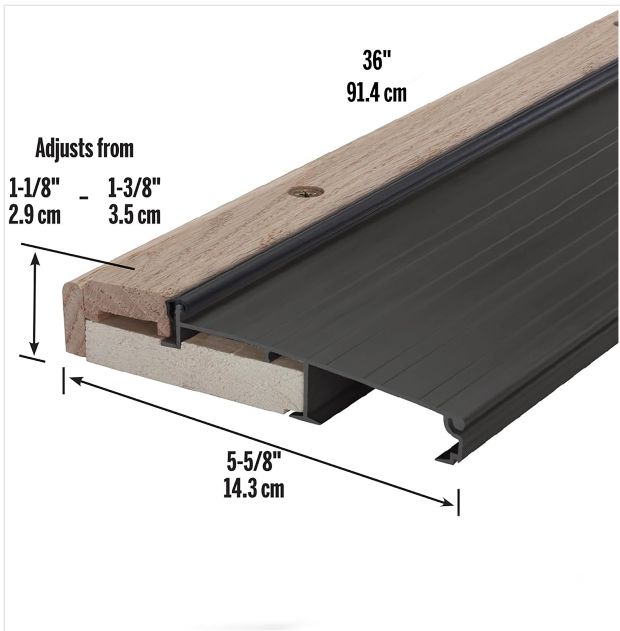
Figure 2: Threshold dimensions and adjustable height range. The threshold is 36 inches (91.4 cm) long and 5-5/8 inches (14.3 cm) wide. The adjustable riser can be set from 1-1/8 inches (2.9 cm) to 1-3/8 inches (3.5 cm) in height.
