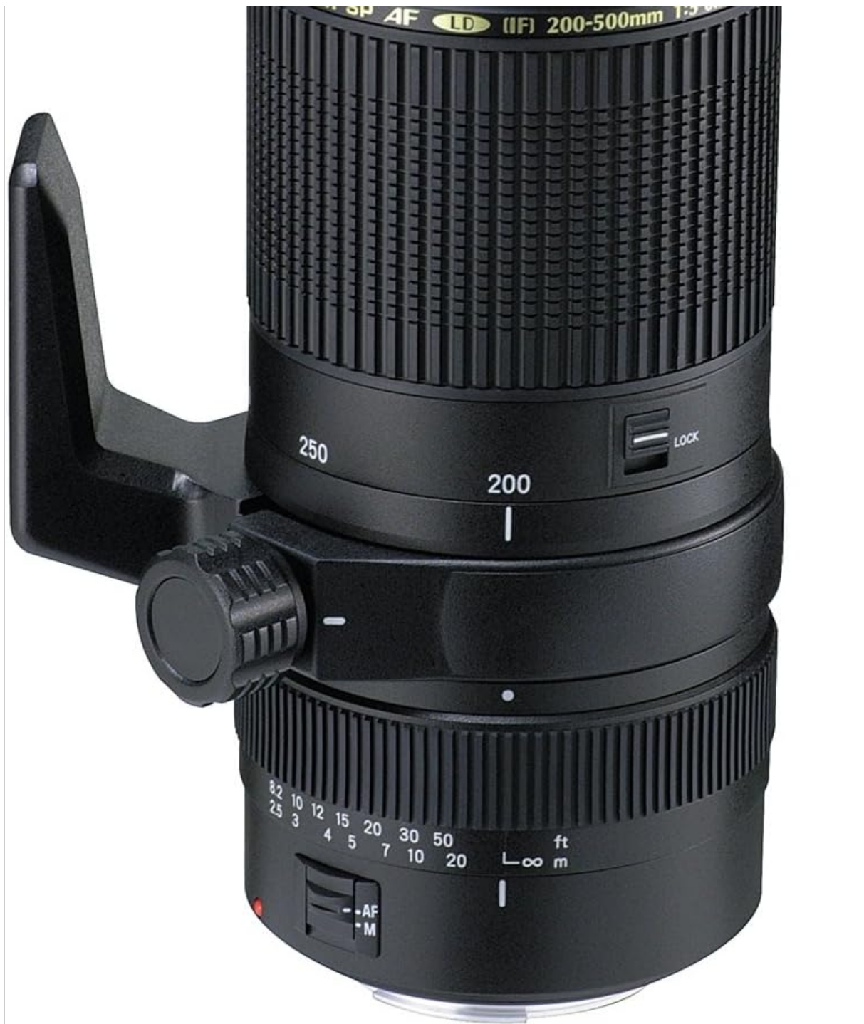
Figure 2: Detail of the AF/M switch and focus distance scale. The switch allows selection between Autofocus (AF) and Manual Focus (M). The focus distance scale shows distances in feet (ft) and meters (m).
