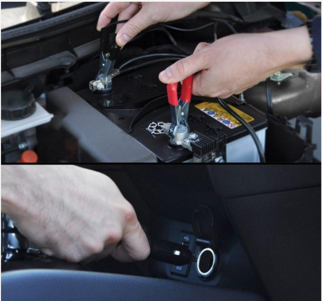
Image 5.1: Illustration of connecting the charger using battery clamps and the 12V DC plug.
