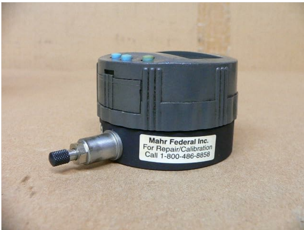
Figure 2: Side view of the indicator, showing the mounting stem and the product label with manufacturer information.
