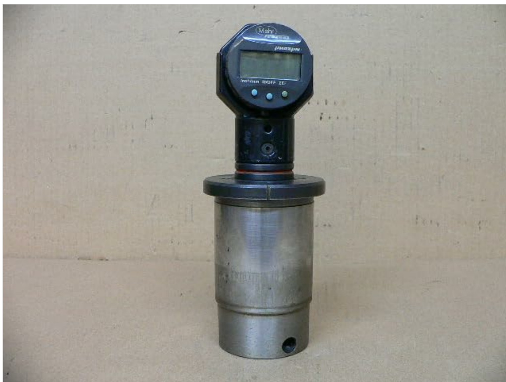
Figure 1: Front view of the Mahr Federal uMaxum Digital Electronic Comparator Indicator, showing the digital display and control buttons.
