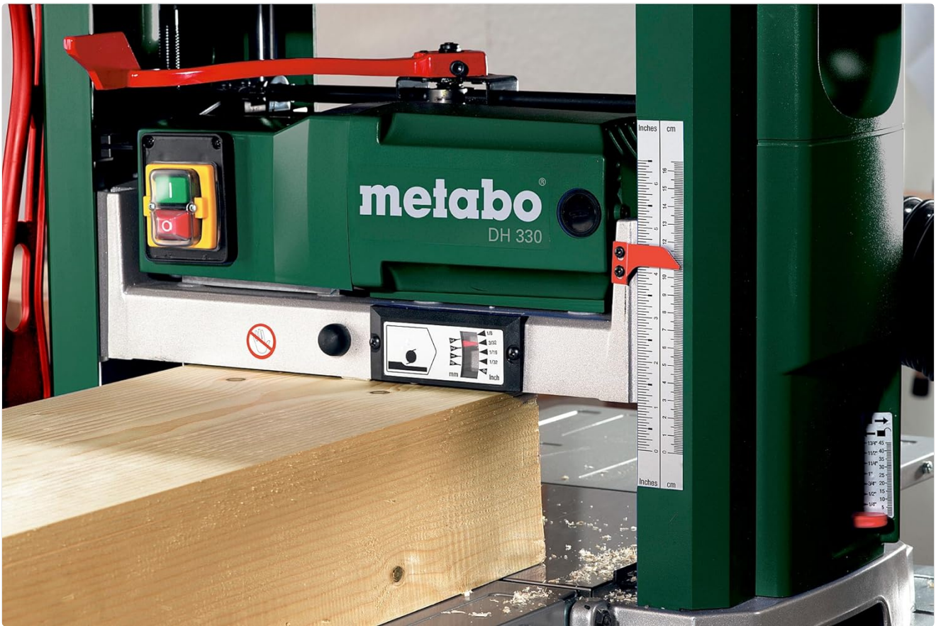
Figure 4: Close-up view of the depth adjustment scale and crank handle on the Metabo DH 330, showing precise measurement markings.
