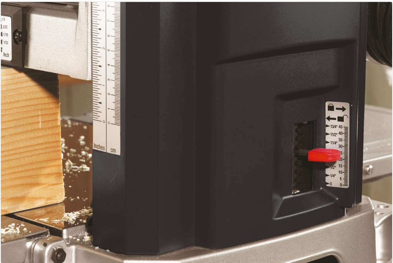
Figure 5: Detail of the planer lock mechanism on the Metabo DH 330, used to secure the planing depth setting.
