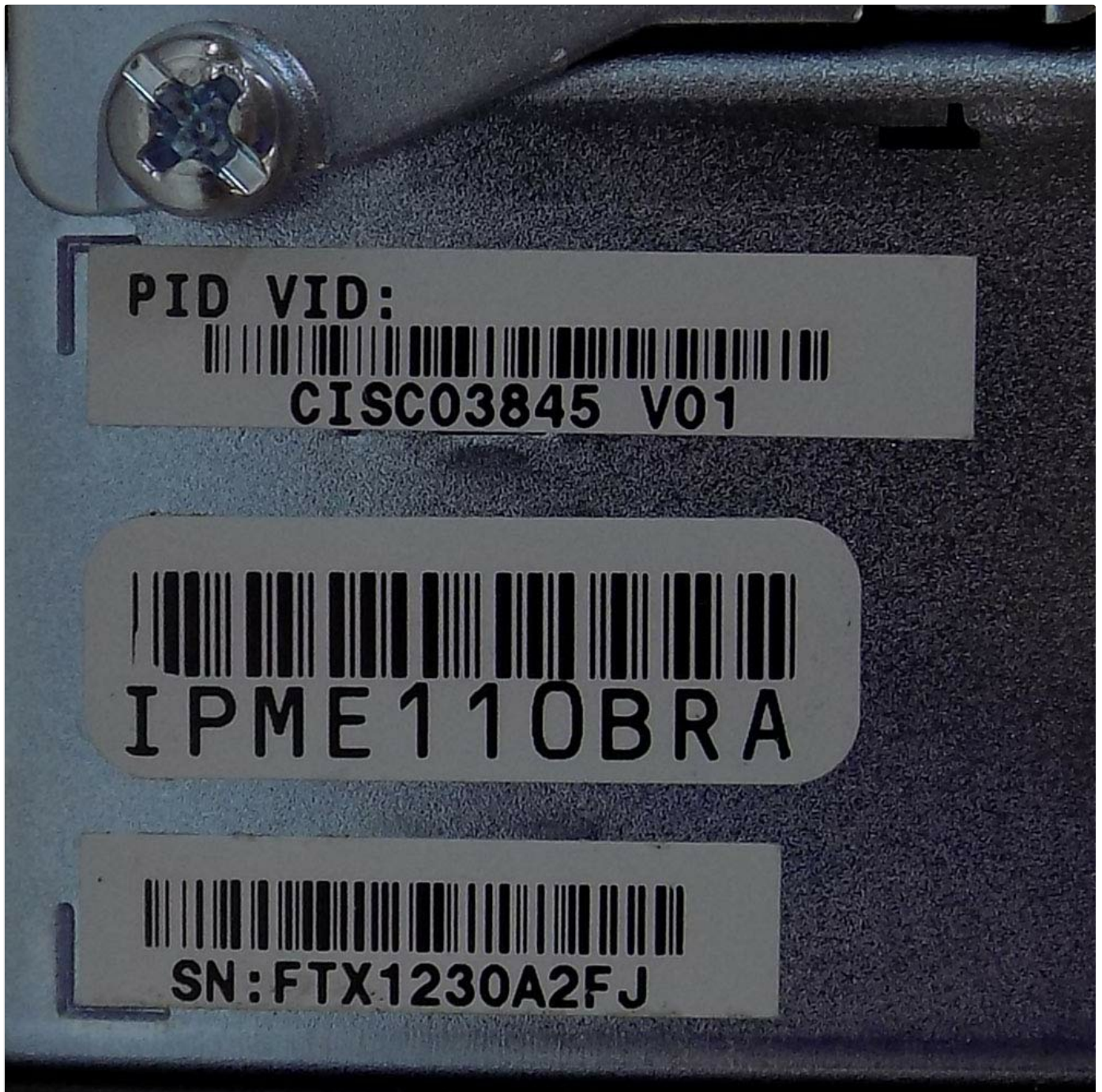
Figure 2.4: Close-up view of the Product ID (PID), Vendor ID (VID), and Serial Number (SN: FTX1230A2FJ) labels on the Cisco 3845.
