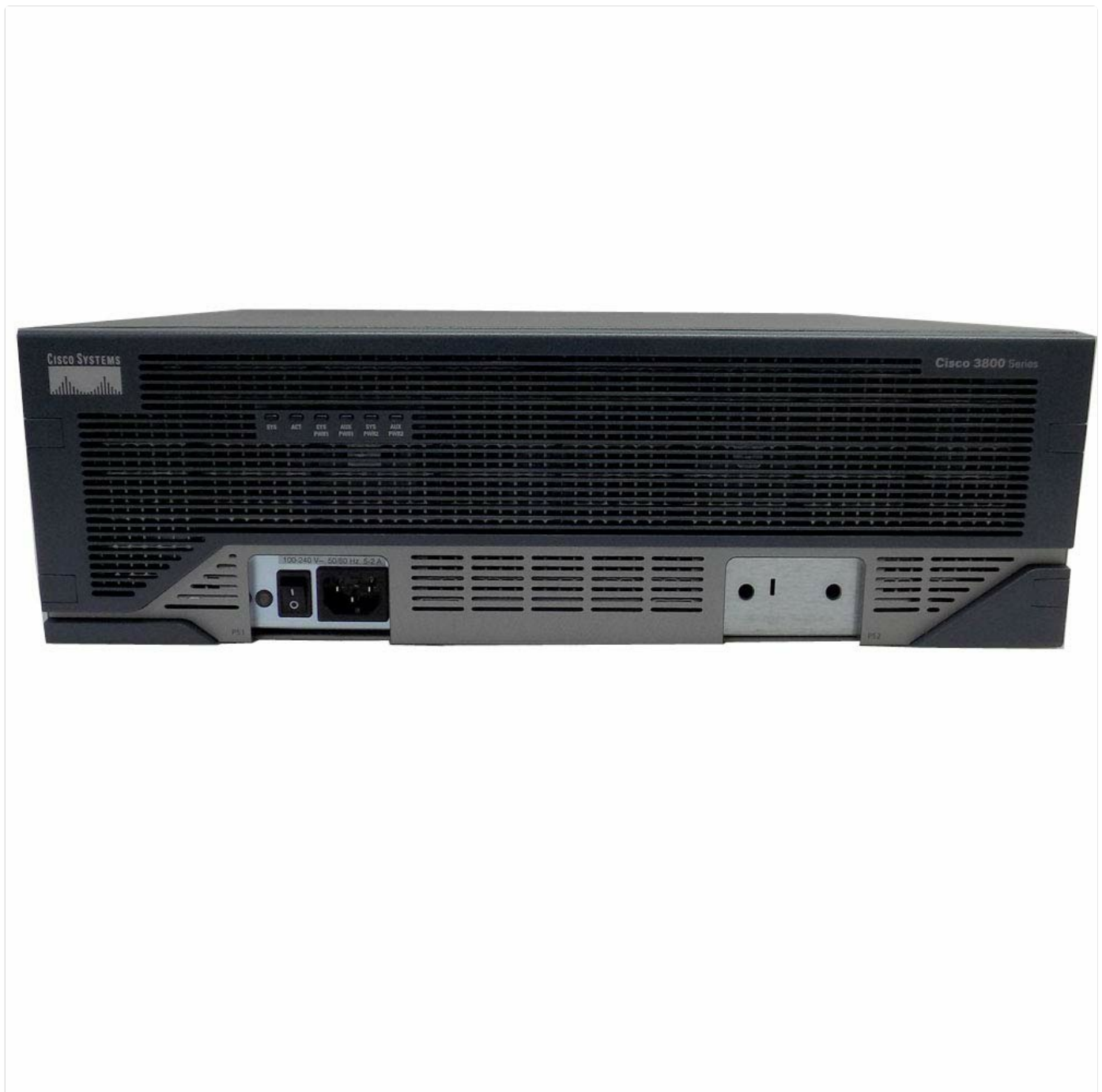
Figure 2.5: Rear view of a Cisco 3800 Series router, illustrating the power input port and ventilation grilles for heat dissipation.
