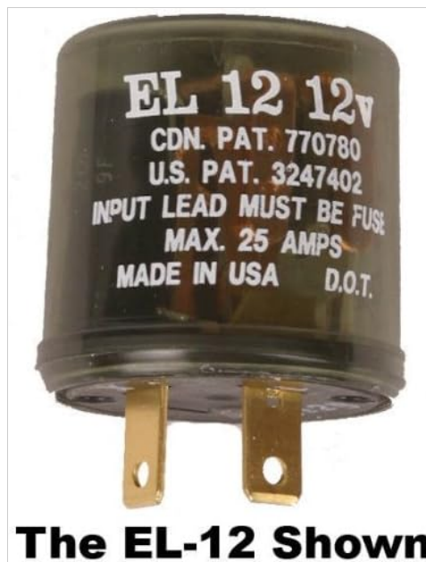
Image 2: Close-up of the Novita EL12 Flasher, highlighting its model number and electrical specifications.
