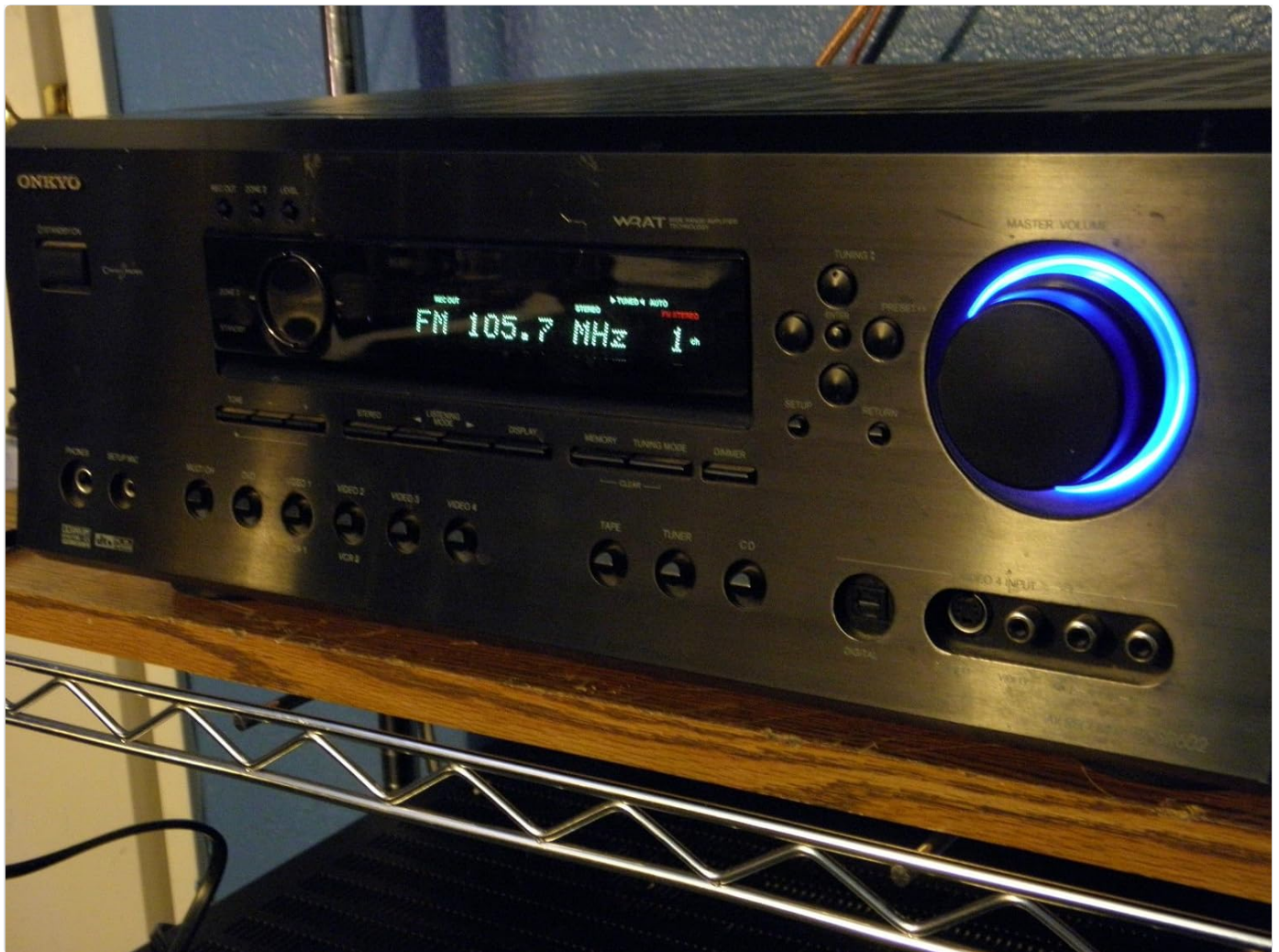
Figure 1.1: Front panel of the Onkyo TX-SR602 receiver. This image displays the receiver's front panel, featuring the central display, various control buttons for input selection, tuning, and setup, and a prominent master volume knob with a blue LED ring. The display currently shows "FM 105.7 MHz".
