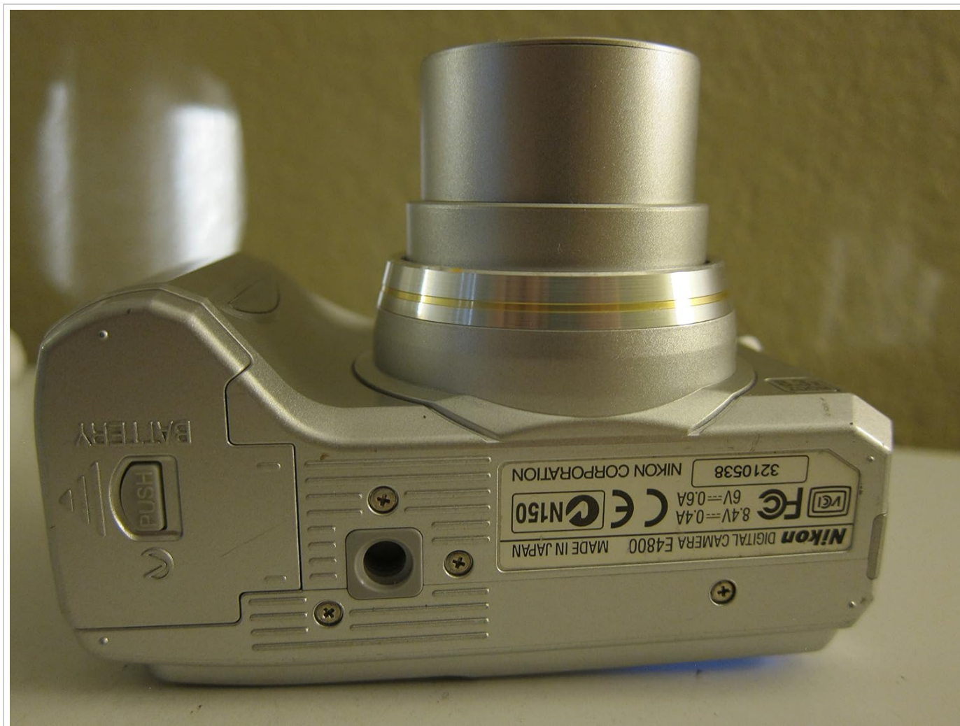
Figure 2: Bottom view of the camera, showing the battery and SD card compartments. The battery is inserted into the larger opening, and the SD card into the smaller slot.
