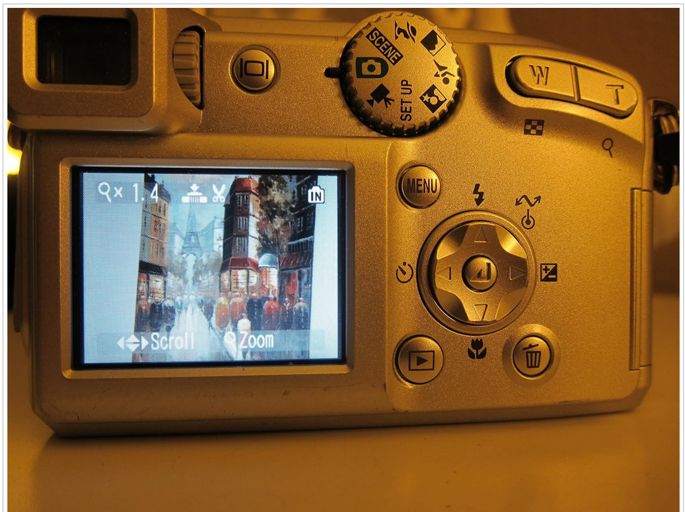
Figure 6: The camera's LCD screen displaying a zoomed-in image, demonstrating the playback and review functions.
