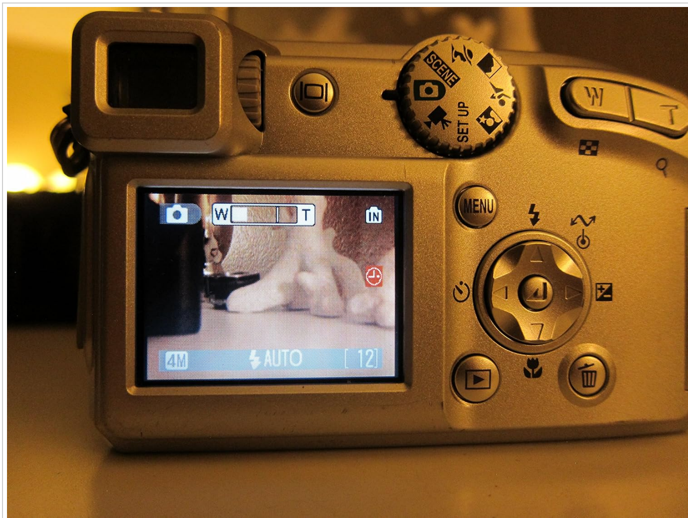
Figure 5: Rear view of the camera, showing the LCD monitor and the mode dial for selecting various shooting settings.
