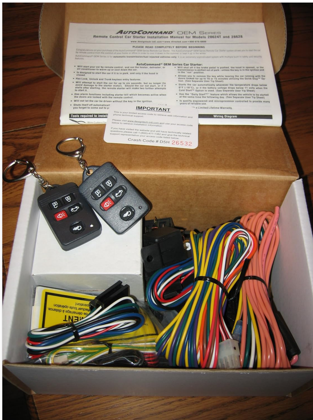
Image 2: Contents of the AutoCommand car starter kit. The image shows two remote control key fobs, various colored wiring harnesses bundled together, and an instruction manual or installation guide visible inside the box. This illustrates the components included for installation.
