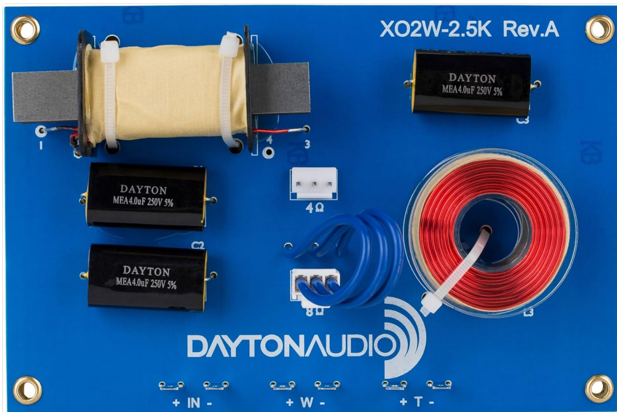
Image: The Dayton Audio XO2W-2.5K speaker crossover board, showing input, woofer, and tweeter terminals, along with inductors and capacitors. The board is blue with white markings.
