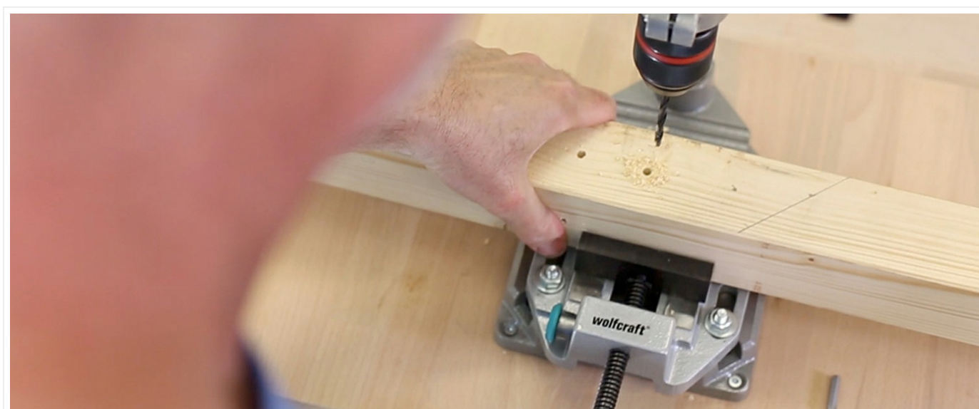
Image 6: A user operating the drill stand to drill into a piece of wood, which is securely held by a clamp on the base plate.
