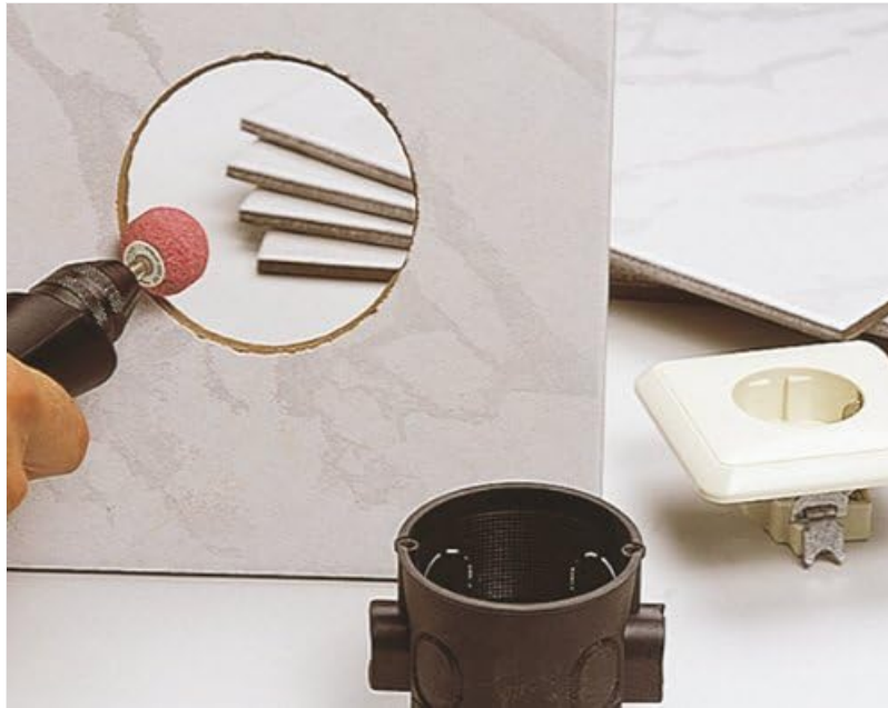
Figure 3: Example of a mounted stone in use, smoothing a circular opening in a workpiece, demonstrating its application for precise shaping.
