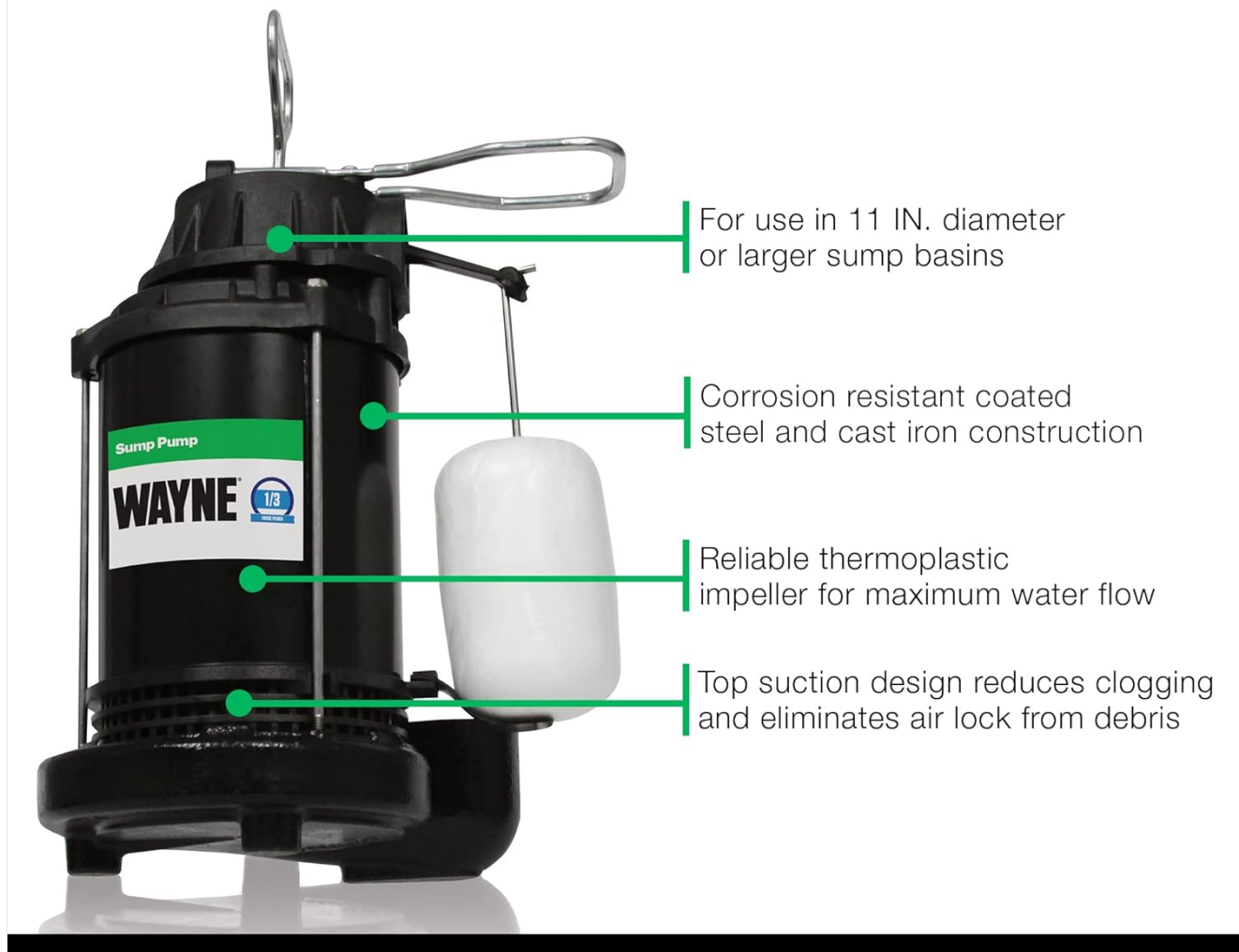
Figure 3: Detailed view of the sump pump's components and design benefits.
