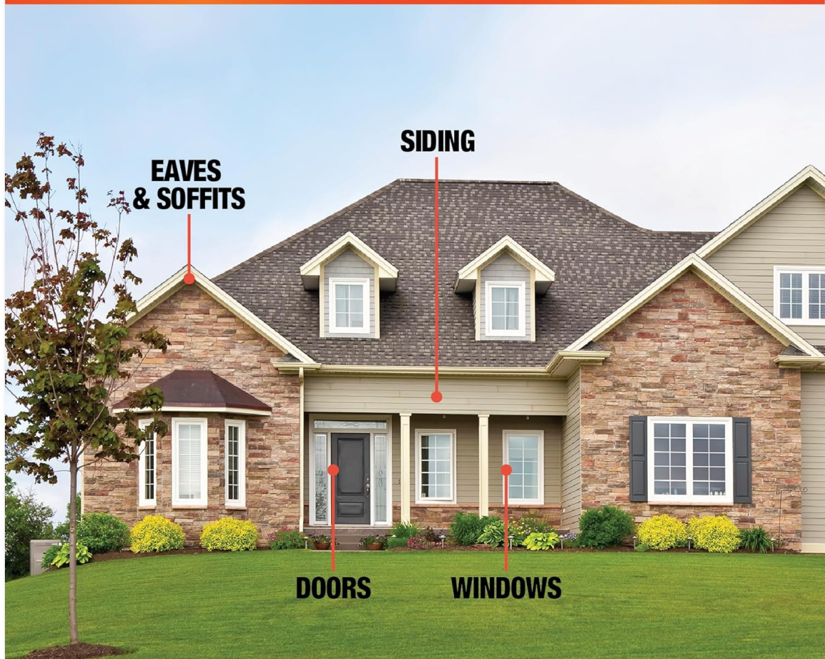
Image 4: An illustration of a house exterior, pointing out common areas where DAP Dynaflex 230 sealant can be effectively applied, such as eaves, soffits, siding, doors, and windows.
