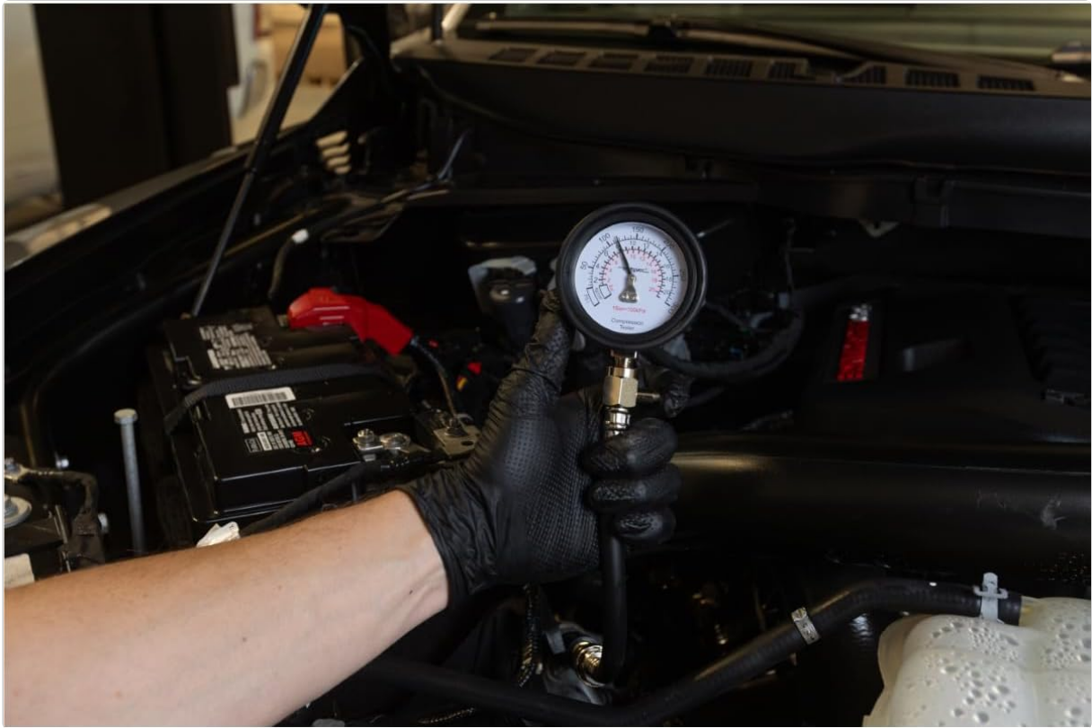
Image: A technician holding the Mityvac compression gauge, connected to a cylinder during a test.
