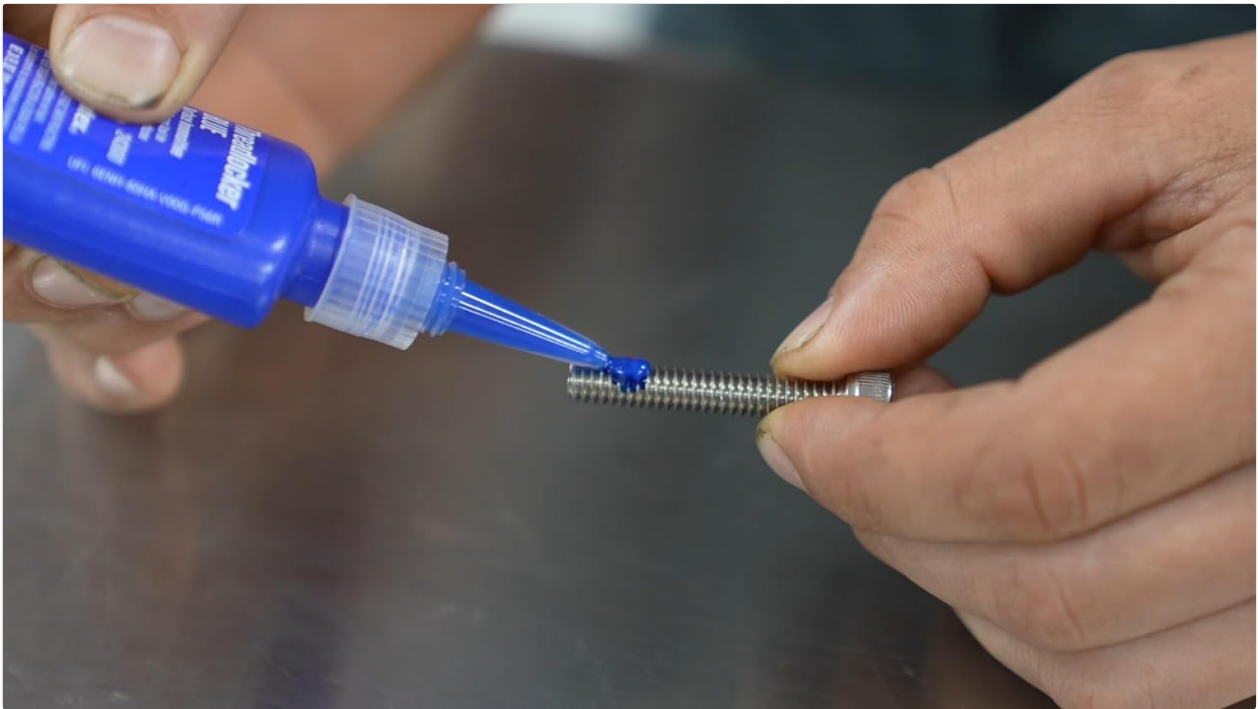
Image: A hand applying a drop of blue threadlocker liquid onto the threads of a metal bolt, demonstrating the application process.
