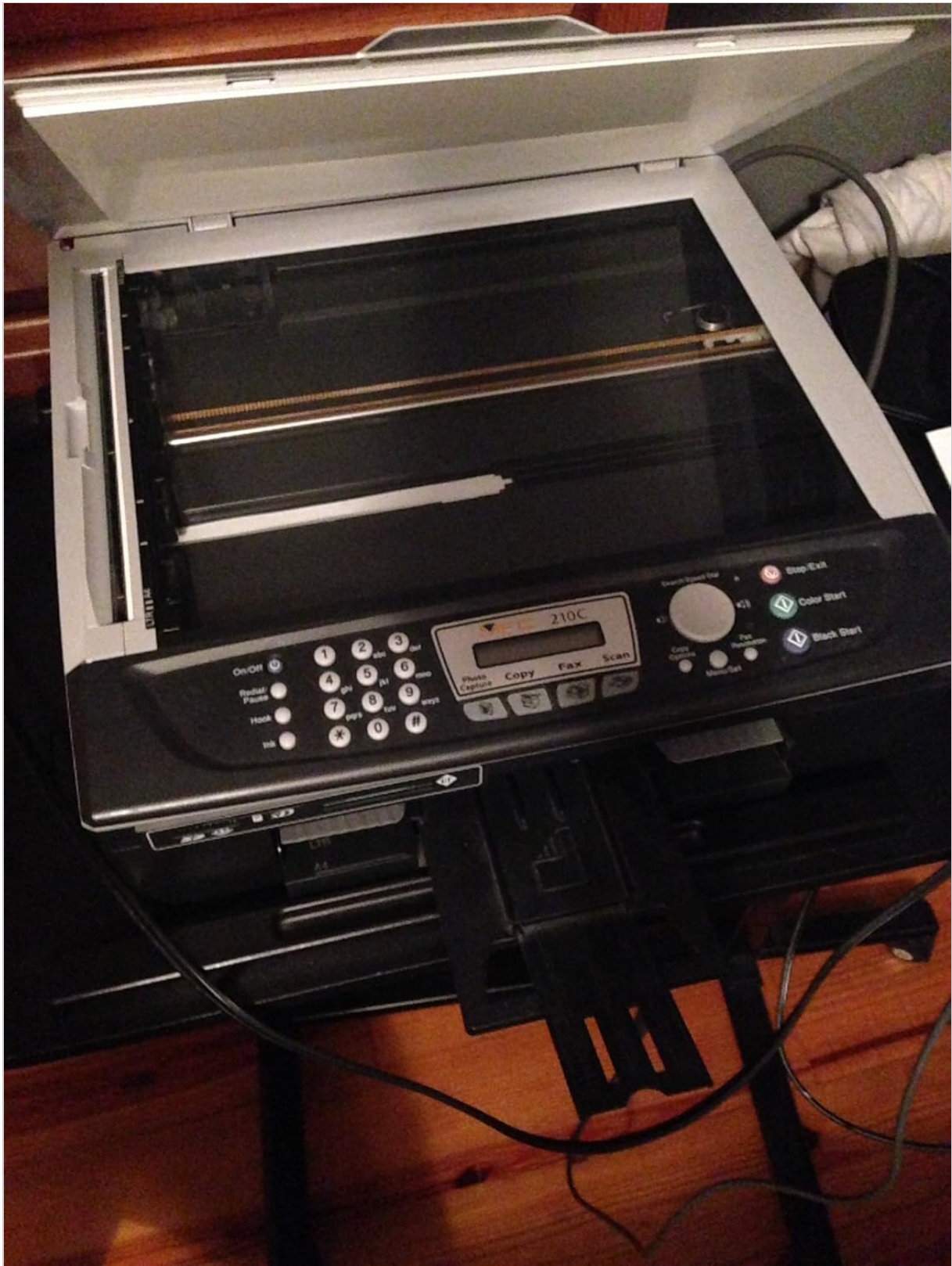
Figure 2: Top view of the Brother MFC-210C Multifunction Printer with the scanner lid open, revealing the scanning glass.
