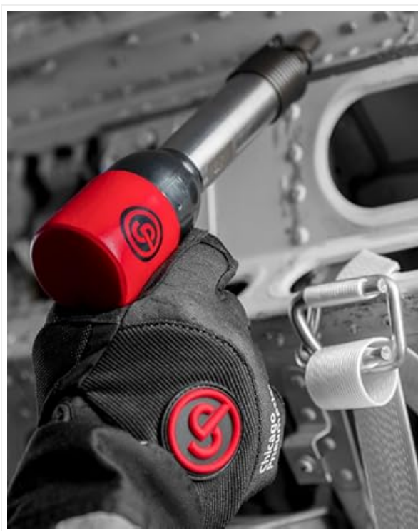
Image: An operator wearing safety gloves using a Chicago Pneumatic cut-off tool to cut metal, demonstrating proper handling.
