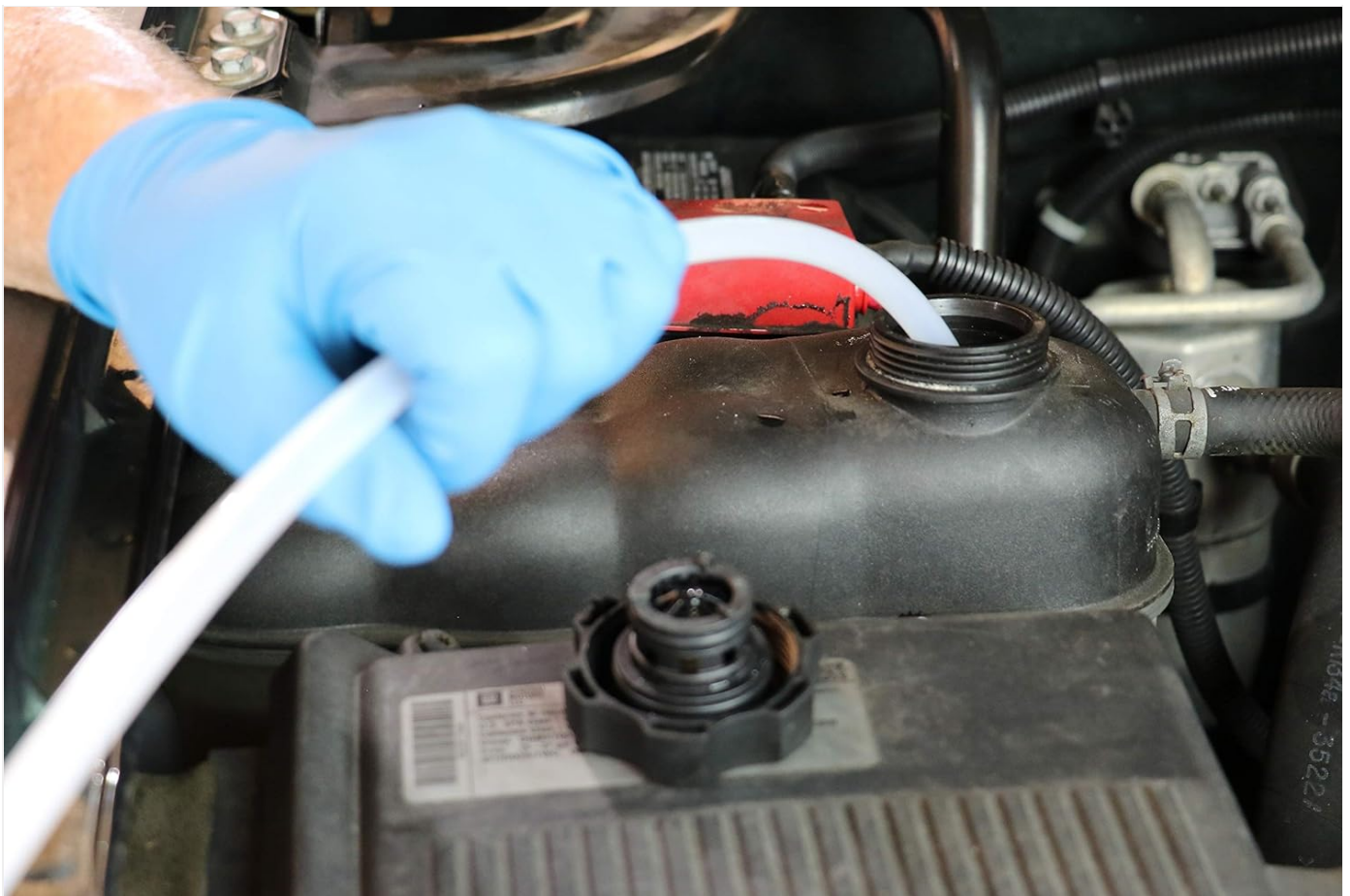
Image 5: A person dispensing fluid from the Mityvac 7201 into a vehicle's coolant reservoir.
