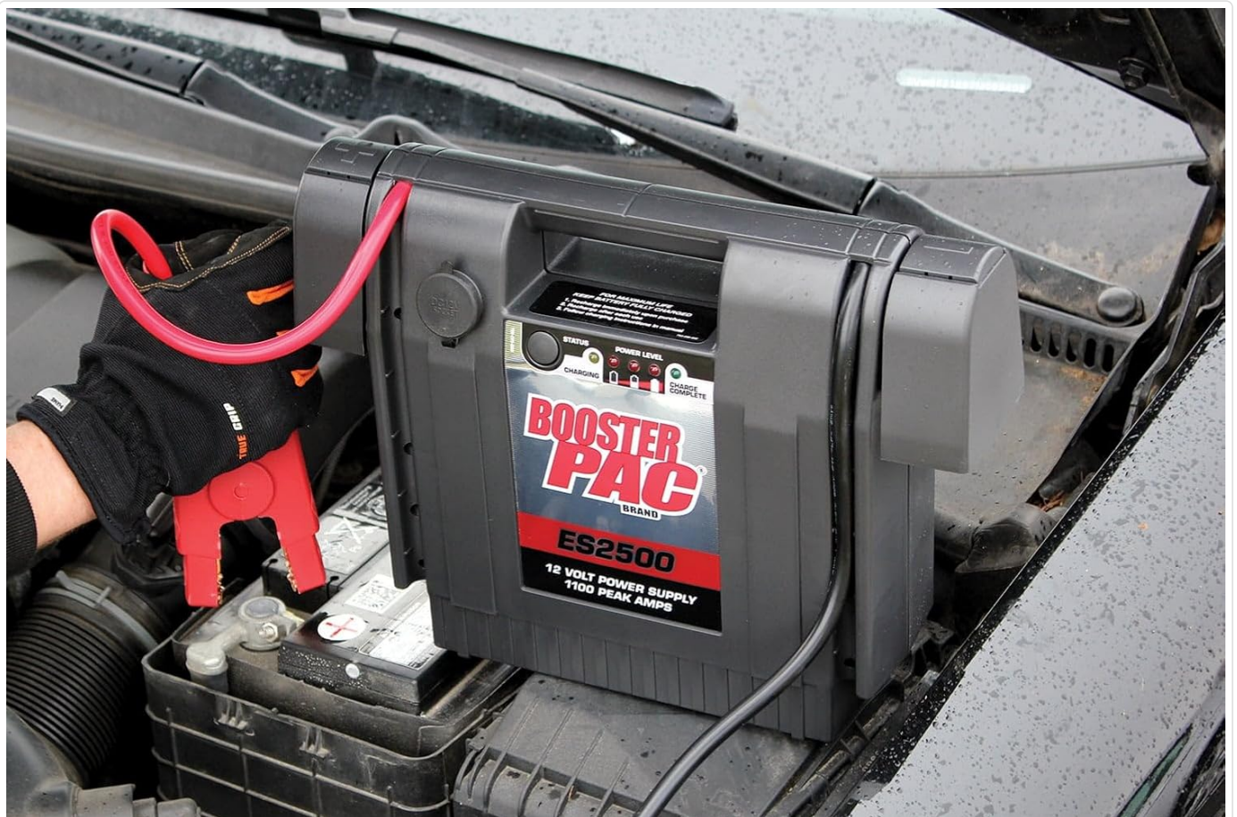
Figure 2: The Booster PAC ES2500 positioned on a vehicle's fender with the red clamp connected to the positive battery terminal.
