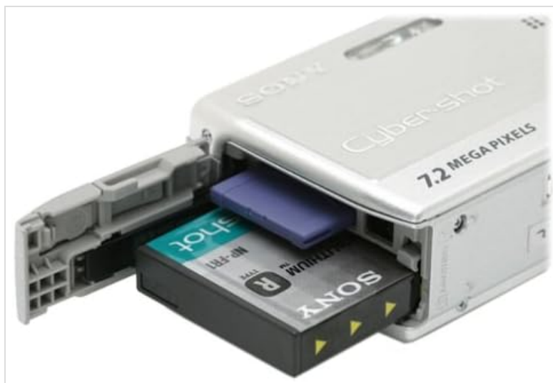
Figure 4: Battery and Memory Stick Compartment. This image illustrates the open compartment on the side of the camera, revealing the slot for the InfoLithium battery and the Memory Stick.
