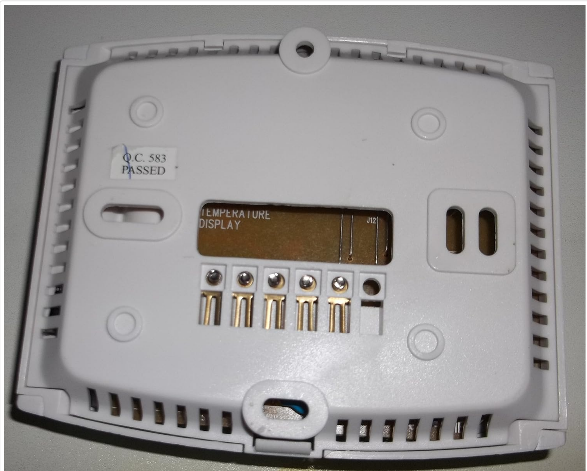
Image: Back view of the Hunter 44110 thermostat, illustrating the wiring terminal block for connecting to your HVAC system.
