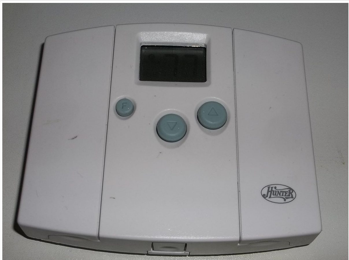
Image: Front view of the Hunter 44110 programmable thermostat, displaying its LCD screen, 'F' (Function) button, and Up/Down arrow buttons for control.
