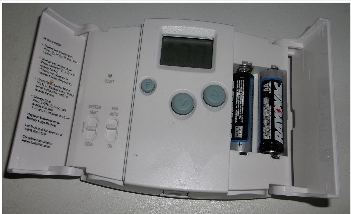
Image: Inside view of the Hunter 44110 thermostat, showing the battery compartment with two AA batteries installed, alongside basic operational instructions printed on the unit.
