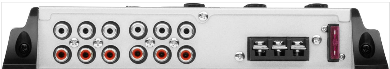
Figure 4.3: Rear View of the BX35 Crossover. This image shows the rear panel of the BX35, detailing all RCA input and output connections, the power terminal block (12V+, REM, GROUND), and the fuse holder. This is crucial for understanding wiring connections.
