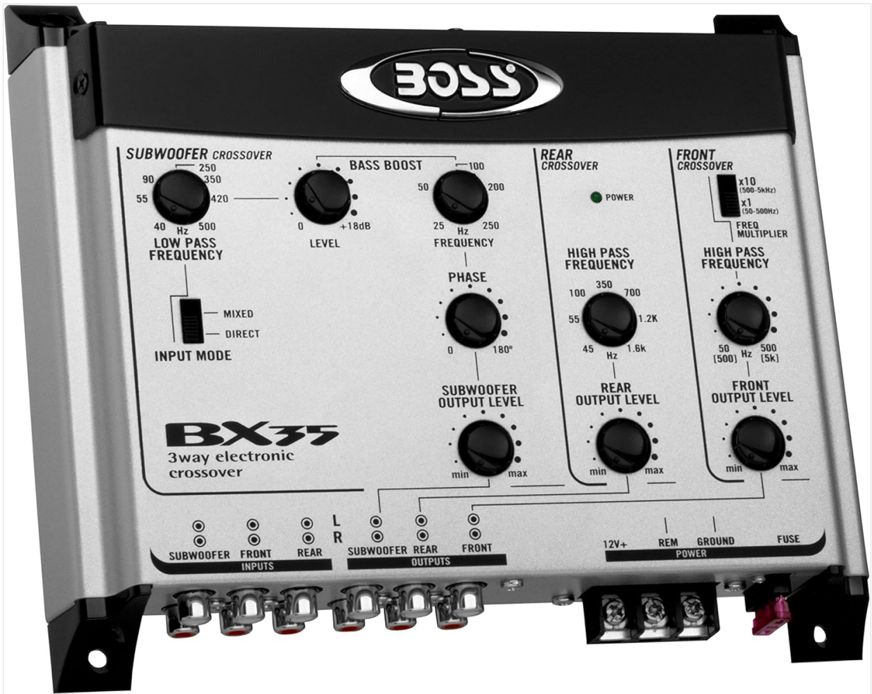
Figure 4.2: Angled View of the BX35 Crossover. An angled perspective of the BX35, highlighting the layout of the control panel and the robust casing. This view provides a clearer look at the input mode switch and the various frequency and level adjustment knobs.
