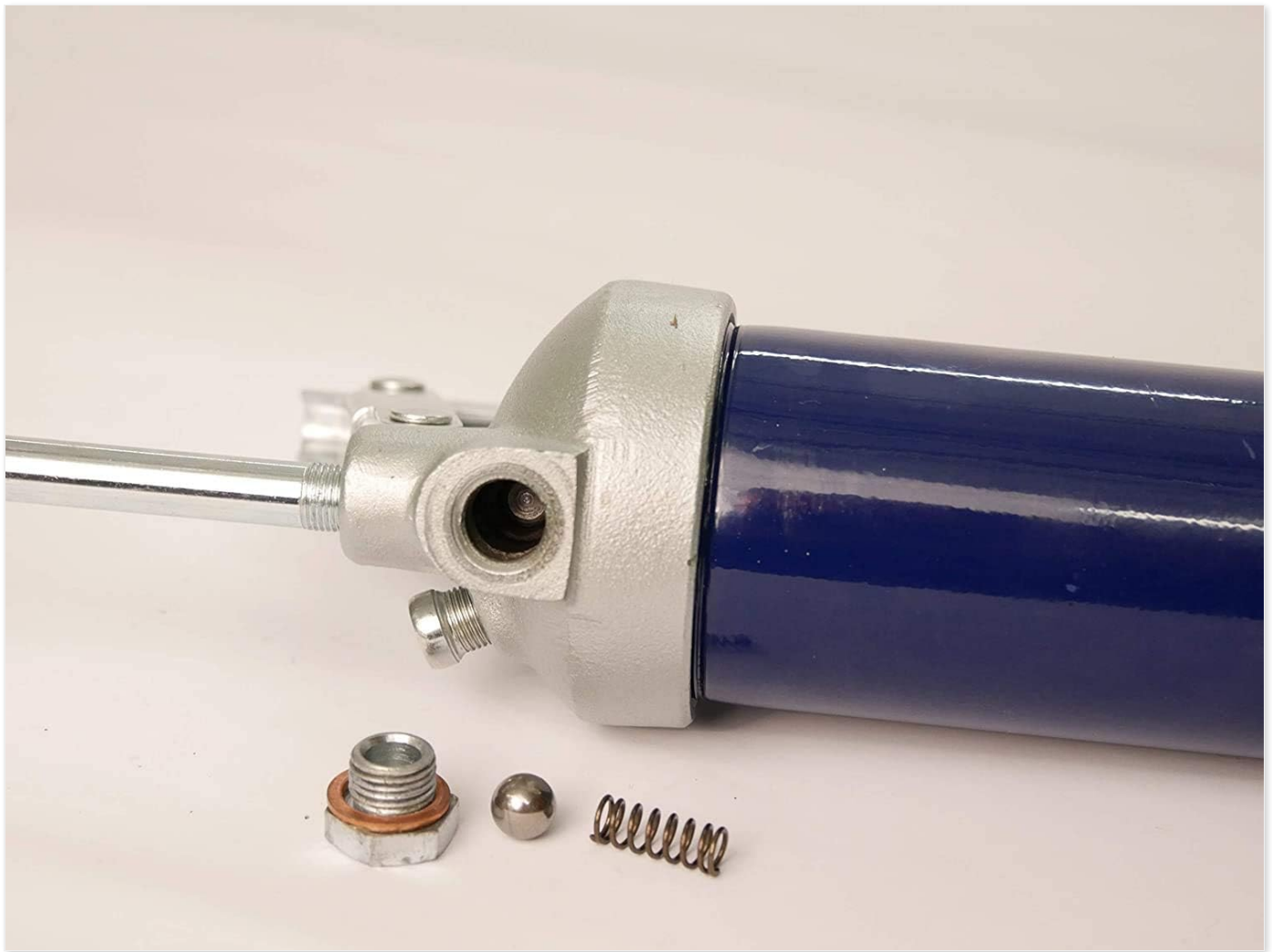
Image: A close-up view of the grease gun's head assembly, showing the accessible check valve and its components (nut, ball bearing, spring) for maintenance.
