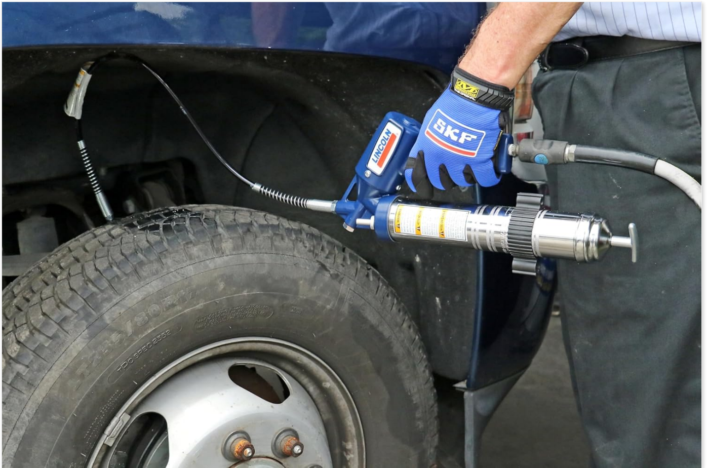
Image: A person wearing gloves using a Lincoln grease gun to lubricate a component near a vehicle wheel, demonstrating practical application.
