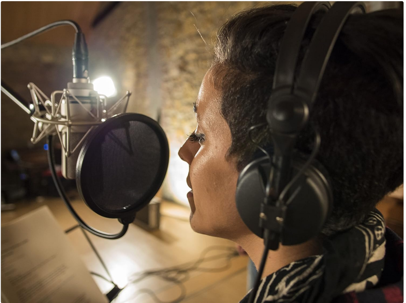
Figure 5.1: Proper microphone technique for vocal recording, showing a user speaking into the Neumann TLM 103-MT with a pop filter to reduce plosives.
