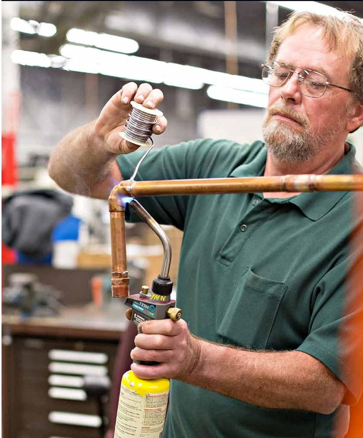
Figure 2: Proper use of the TurboTorch TX504 for soldering applications.
