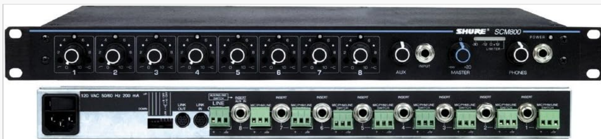
Image: Front and rear panels of the Shure SCM800 Eight Channel Microphone Mixer. The front panel shows eight input level controls, an auxiliary input, master level, limiter indicator, and headphone output. The rear panel displays power input, link connections, and eight microphone/line inputs with phantom power switches.
