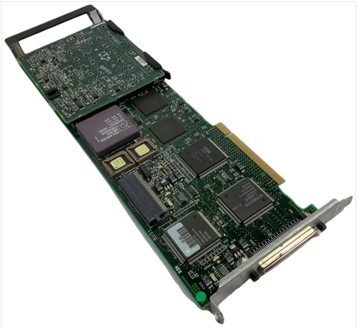
Figure 1: Front view of the Compaq 2-port SCSI Controller. The image displays the green circuit board with various integrated circuits, connectors, and the PCI interface edge connector. The metal bracket for securing the card in a computer chassis is visible on the right side, along with the external SCSI port.
