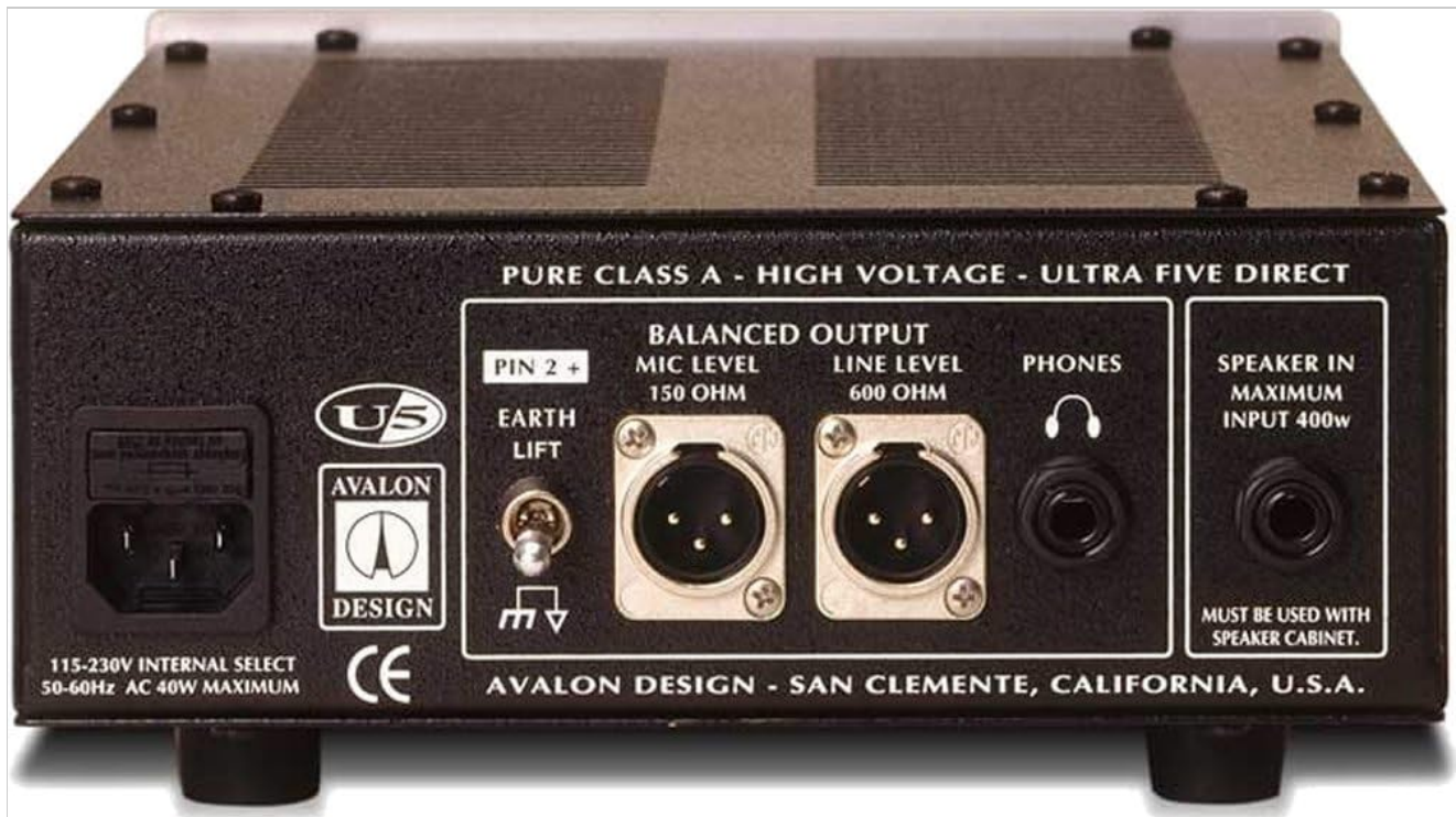
Figure 2: Rear Panel Connections of the Avalon U5
