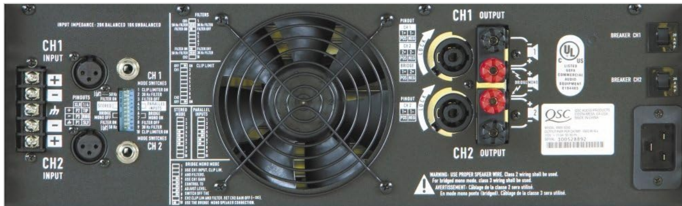
Figure 3.1: Rear panel of the QSC RMX5050 Power Amplifier. This image highlights the various input options (XLR, TRS, barrier strip), output connectors (Speakon, binding posts), DIP switches for configuration, and the AC power inlet.
