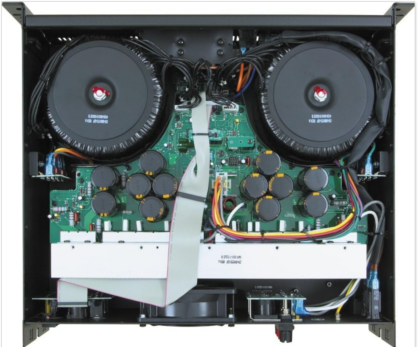
Figure 5.1: Internal view of the QSC RMX5050 Power Amplifier. This image shows the large toroidal transformers, circuit boards, capacitors, and the central cooling fan, emphasizing the robust internal design and the importance of clear airflow.
