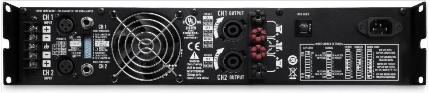
Figure 3.1: Rear view of the QSC RMX1450a Stereo Power Amplifier. This image highlights the various input and output connectors, including XLR, 1/4" TRS, barrier strip inputs, and Speakon/binding post outputs, along with mode switches.
