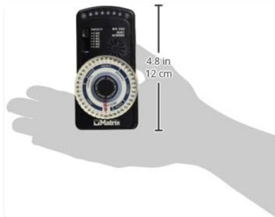
Figure 2: Dimensions of the MATRIX MR800 Tuner Metronome.
