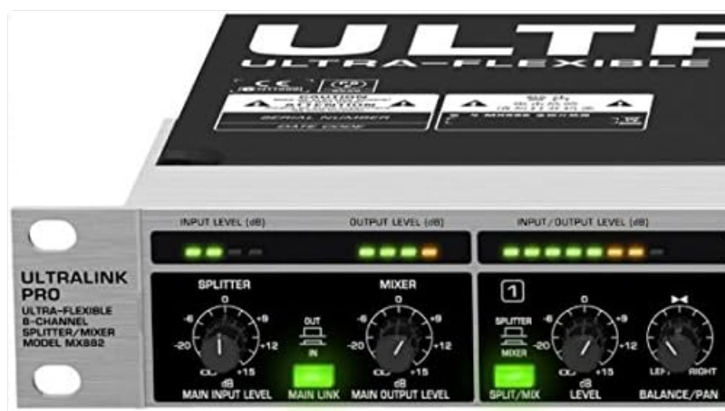
Figure 4.2: Detailed view of the front panel controls for the Behringer Ultralink Pro MX882. This close-up shows the MAIN INPUT LEVEL, MAIN LINK, MAIN OUTPUT LEVEL, SPLIT/MIX switch, LEVEL, and LEFT/RIGHT BALANCE/PAN controls, along with their respective LED meters.
