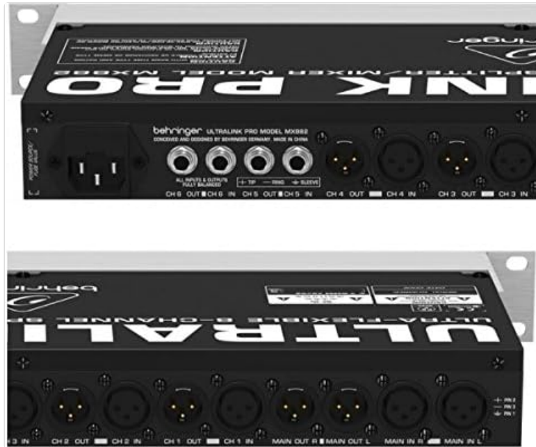
Figure 4.4: Detailed view of the rear panel connections for the Behringer Ultralink Pro MX882. This close-up shows the AC power inlet, XLR inputs and outputs, and 1/4-inch TRS inputs and outputs.
