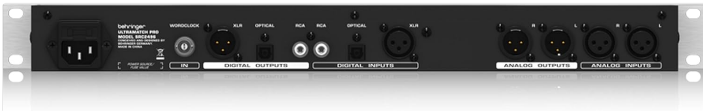
Figure 1: Rear panel connections of the SRC2496. This view shows the power input, wordclock I/O, XLR, RCA, and optical digital inputs and outputs, and XLR analog inputs and outputs.
