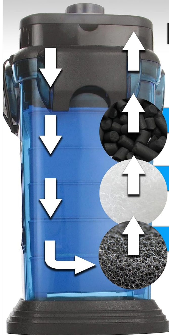
Figure 3: Multi-stage filtration layers: Carbon, Fine Sponge, Coarse Sponge.
