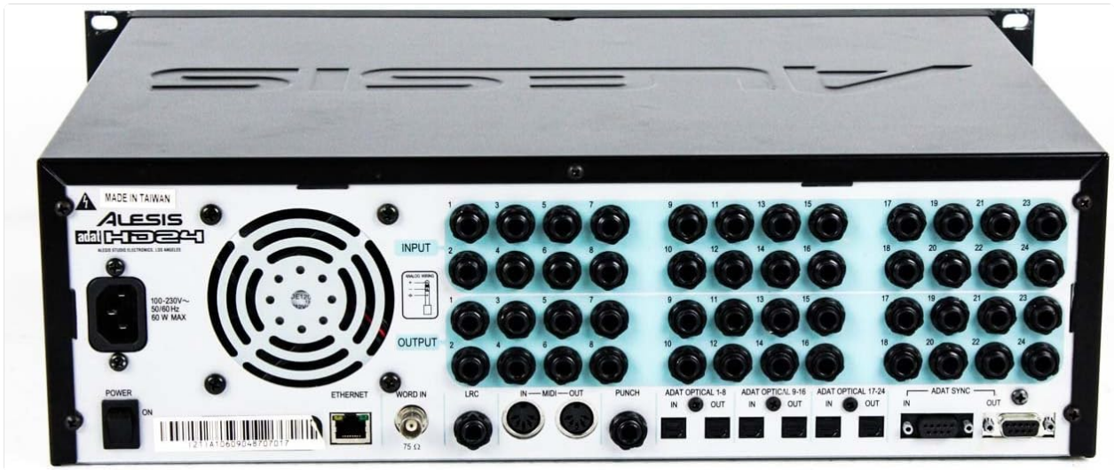
Figure 2.1: Rear panel of the Alesis ADAT-HD24, illustrating the various input and output connections.
