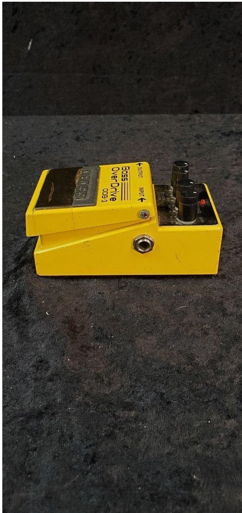
Figure 2: Side view of the BOSS ODB-3, illustrating the input and output jack locations.
