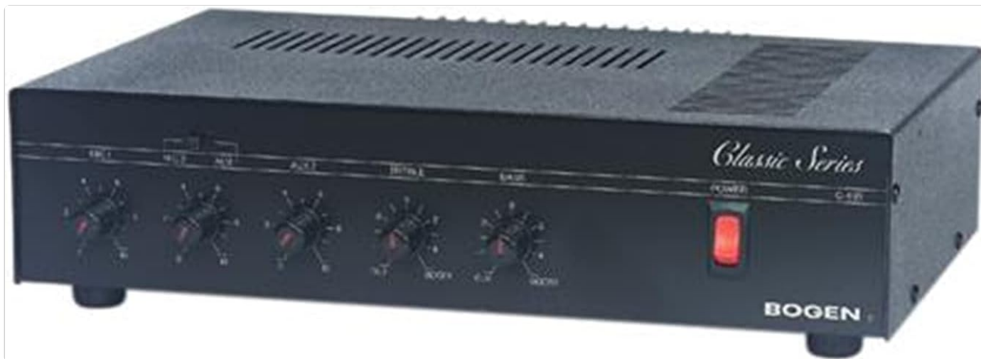
Image 1.1: Front view of the Bogen C100 Classic 100-Watt Amplifier, showing input controls, tone controls, power switch, and Bogen branding.
