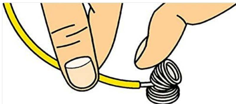
Illustration demonstrating how to connect wires using the spring-wire terminals on the electronic project lab.
