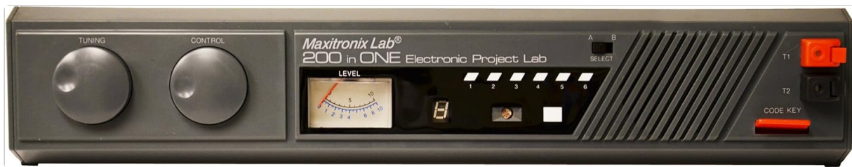
Front panel view of the Maxitronix 200-in-One Electronic Project Lab, showing tuning and control knobs, meter, and LED display.
