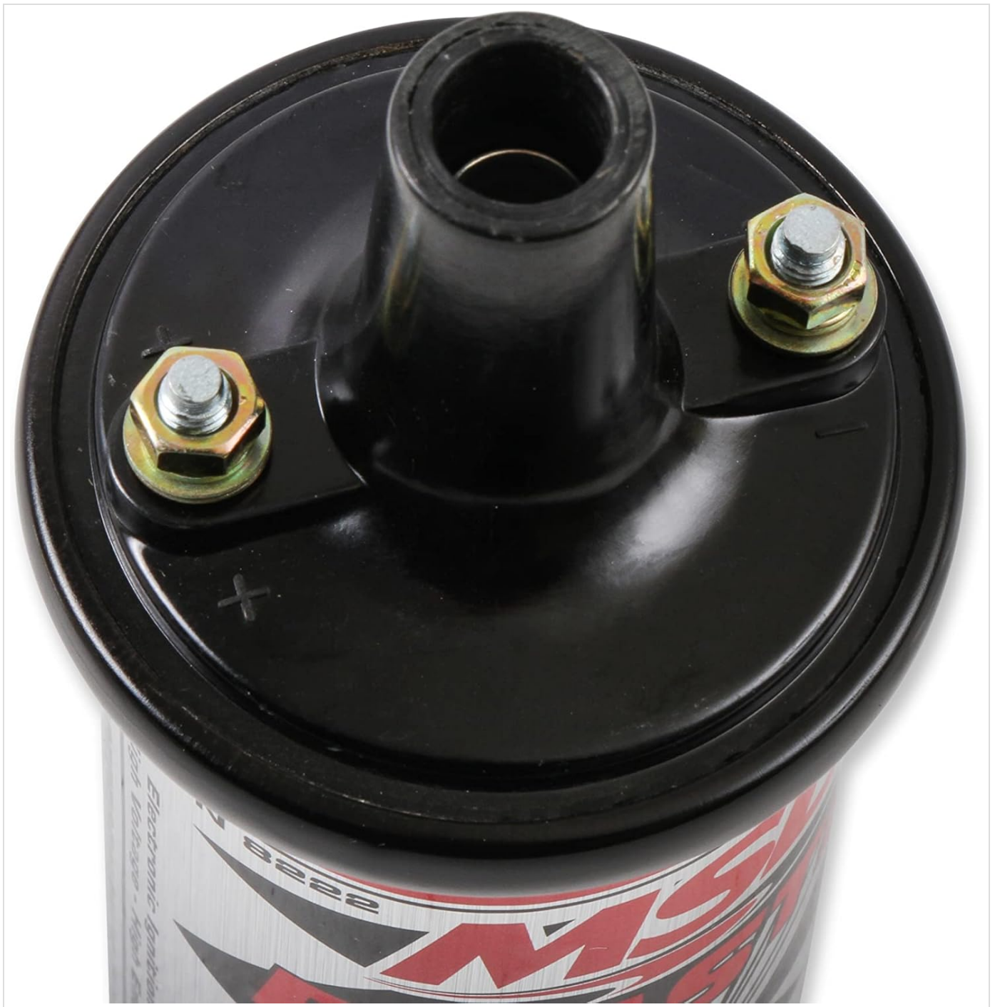
Figure 2: Top view of the MSD 8222 Ignition Coil, showing the positive (+) and negative (-) terminals for primary wiring connections and the central high-tension tower for the spark plug wire.
