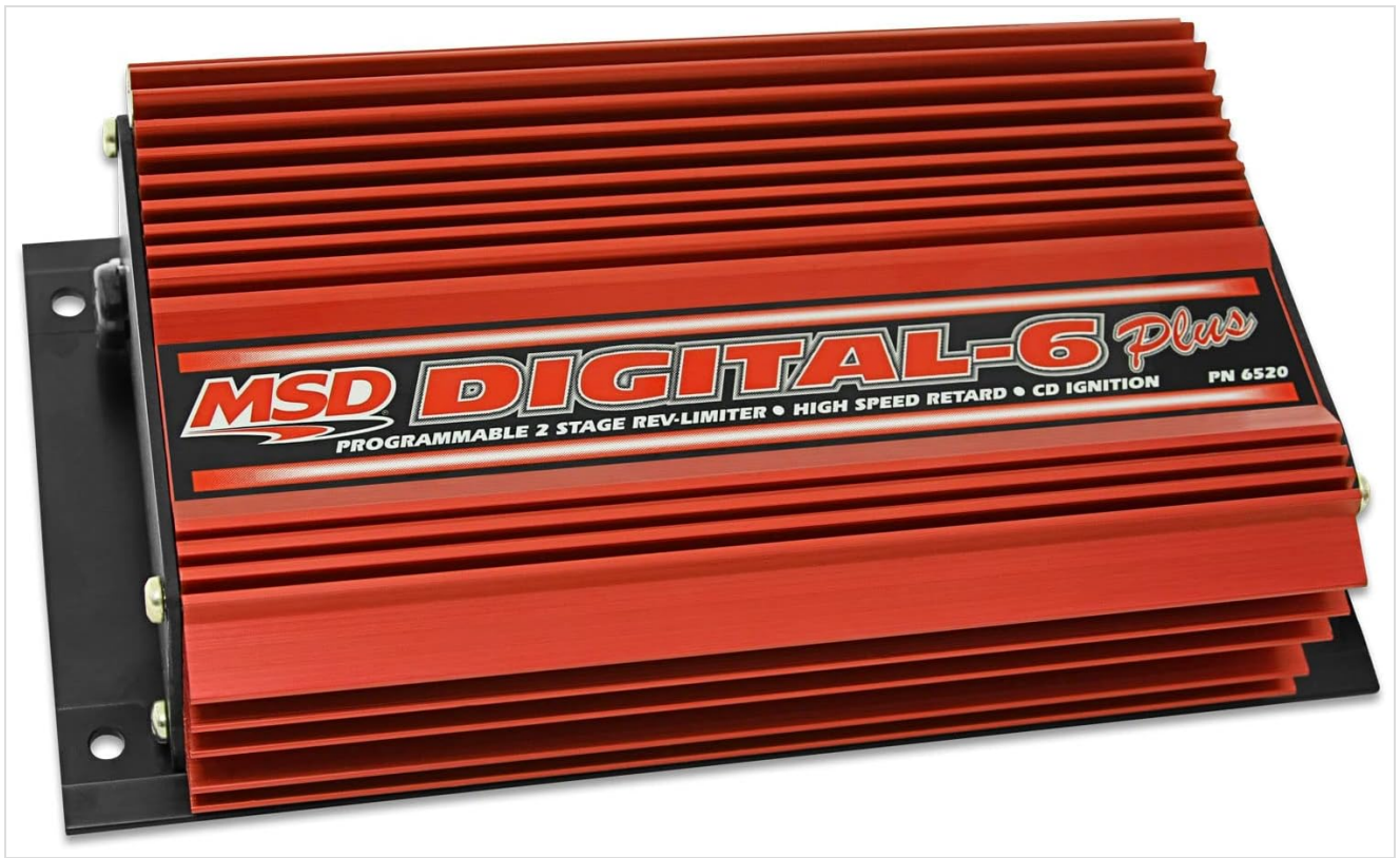
Figure 1: The MSD Digital 6-Plus Ignition Control unit, showing its red finned heat sink design.
