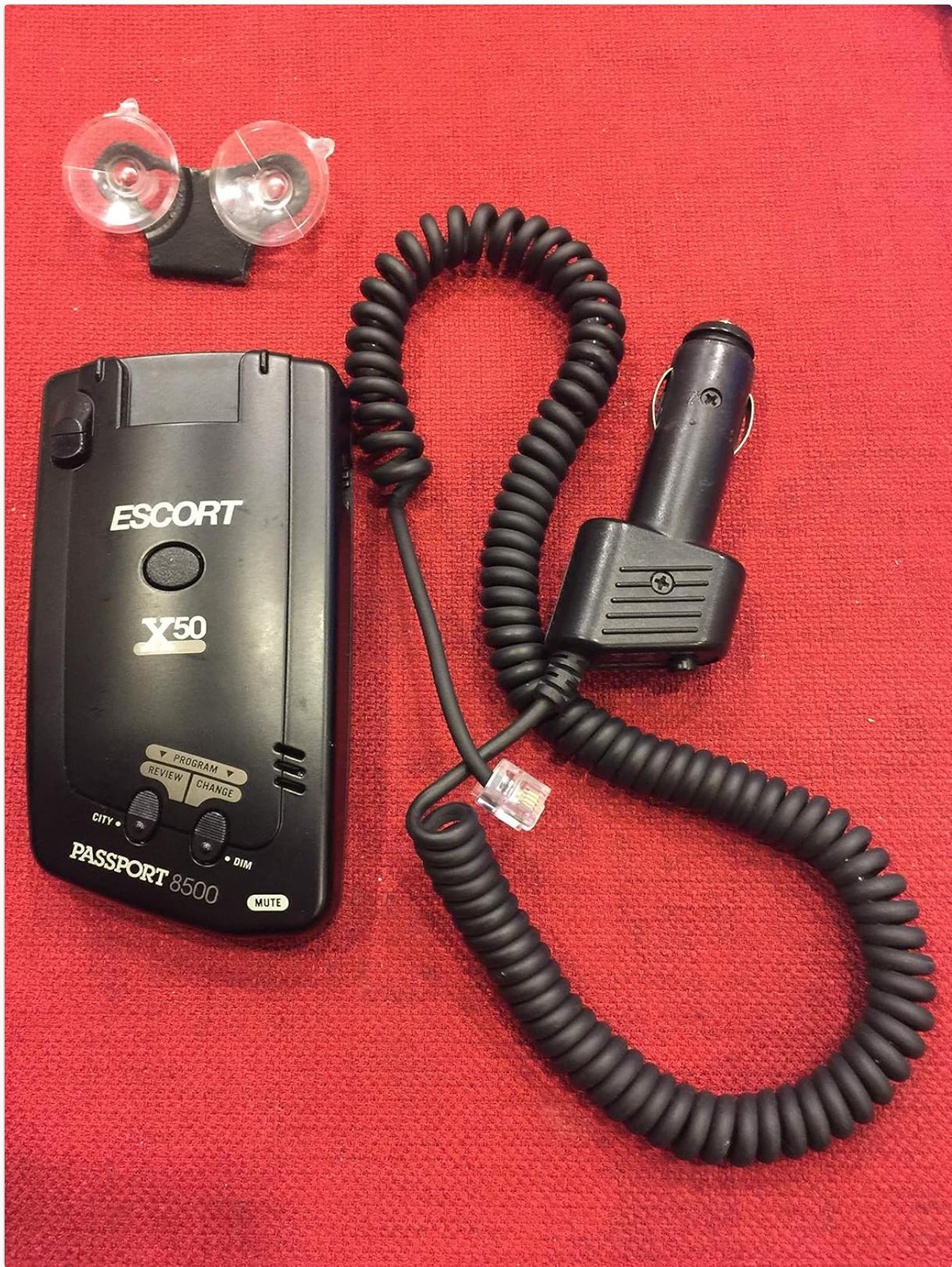
This image displays the Escort Passport 8500 X50 radar and laser detector unit, its suction cup windshield mount, and the coiled SmartCord power cable. The detector unit is black with 'ESCORT' and 'PASSPORT 8500 X50' branding, along with control buttons for 'CITY', 'DIM', 'MUTE', 'PROGRAM', 'REVIEW', and 'CHANGE'. The SmartCord features a cigarette lighter adapter and a coiled cable connecting to the detector.
