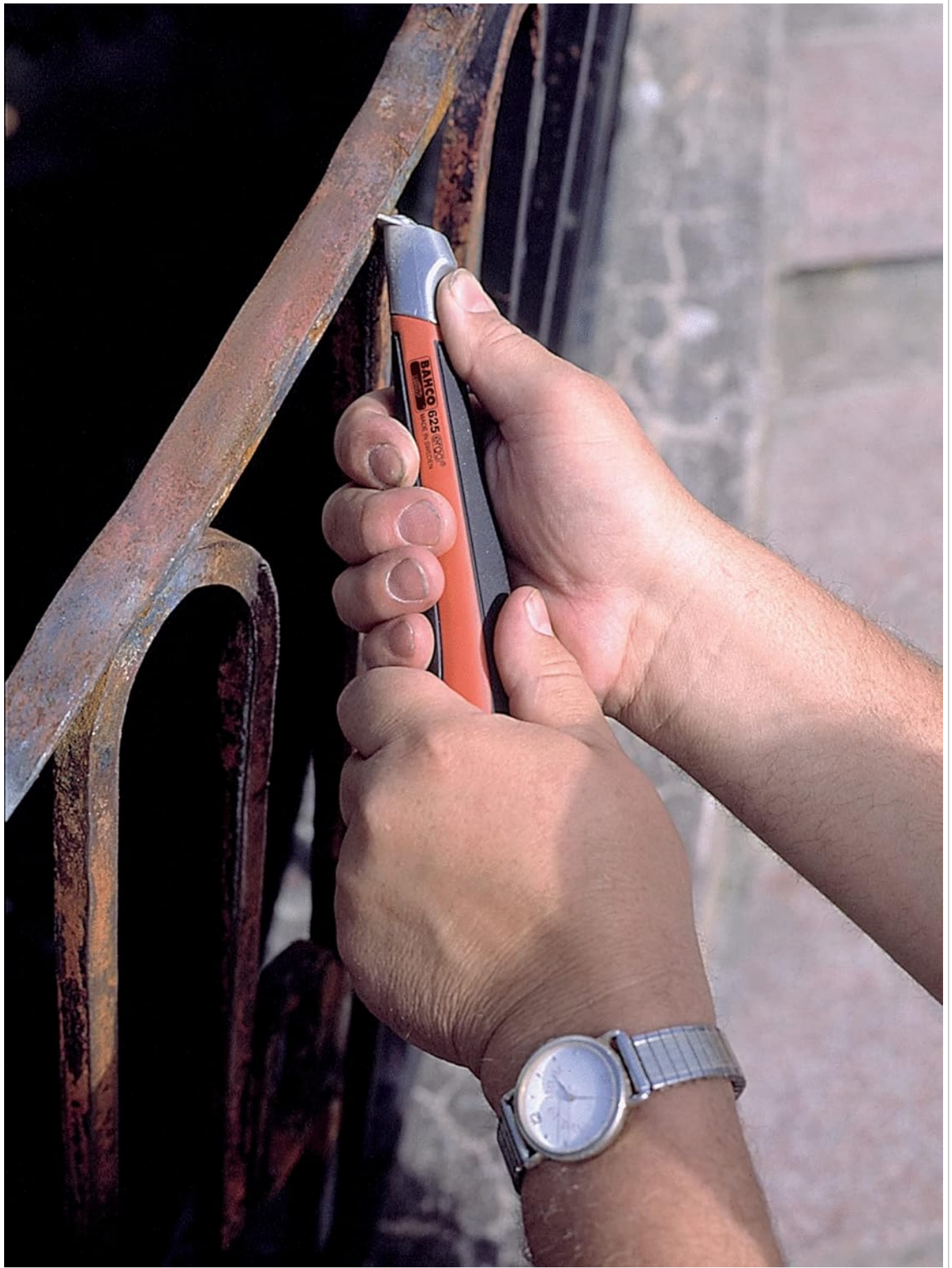
Image 4.1: Demonstrating the Bahco Ergo Pocket Scraper in use for removing rust from a metal surface.
