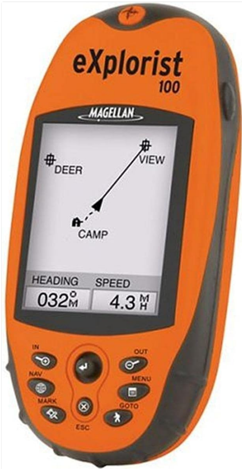
Figure 1: The Magellan eXplorist 100 handheld GPS unit. This image shows the device's front, highlighting its grayscale display, control buttons, and overall ergonomic design. The screen displays navigation information including heading, speed, and a simple map with waypoints labeled "DEER", "VIEW", and "CAMP".
