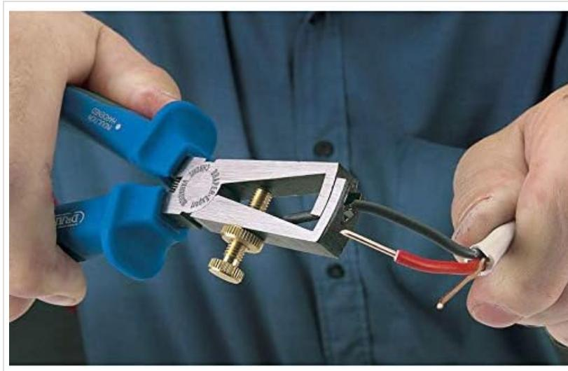
A close-up image demonstrating the Draper Expert Wire-Stripping Pliers in action. A user's hand holds the pliers, which are engaged in stripping the red insulation from an electrical wire, revealing the copper conductor beneath. This illustrates the precise function of the tool.
