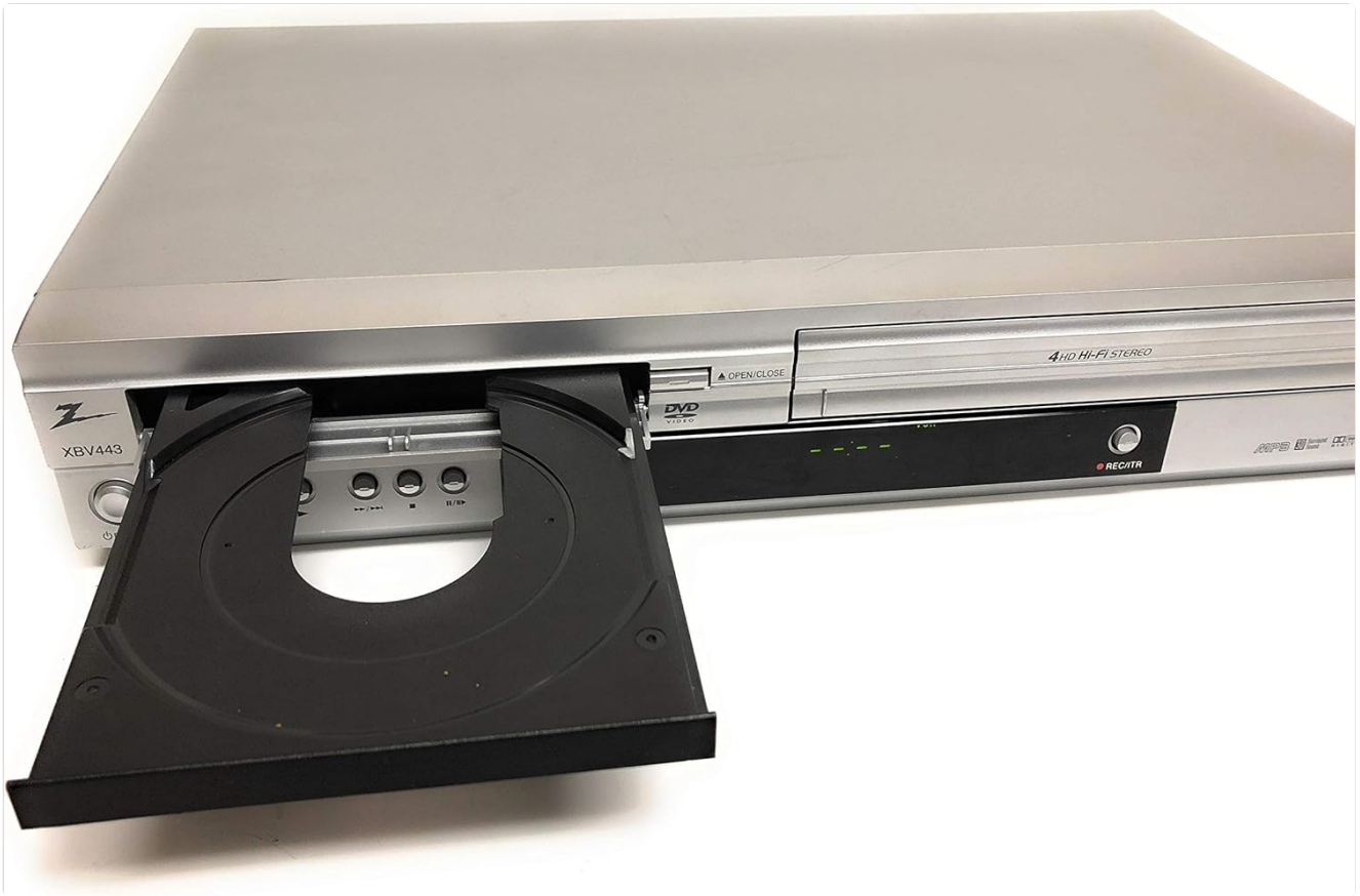
The Zenith XBV443 with its DVD disc tray open, ready for disc insertion.
