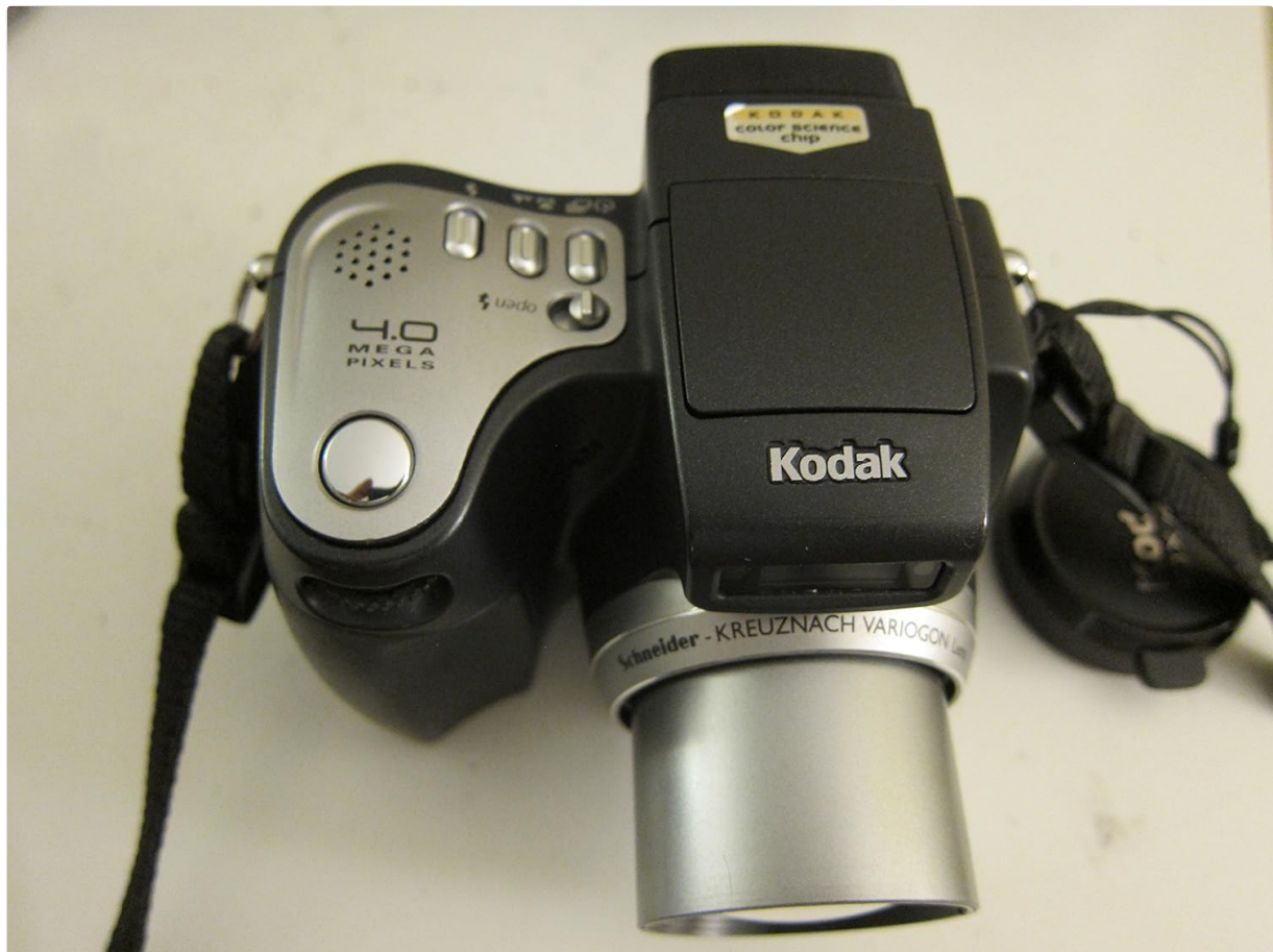
Figure 3.1: Top view of the camera, highlighting the power dial, shutter button, and zoom lever.
