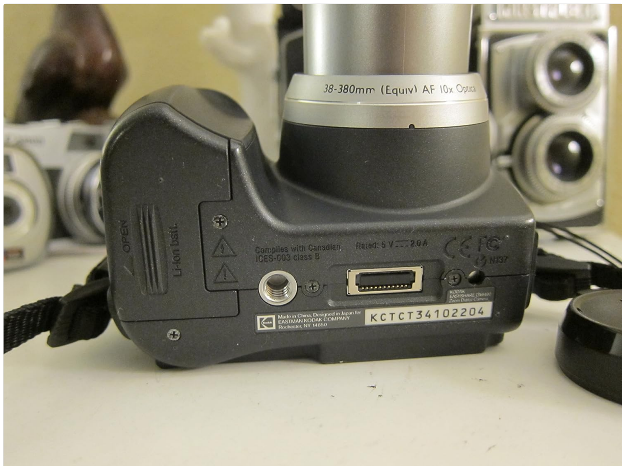
Figure 2.1: The bottom of the camera, showing the battery compartment and various ports.
