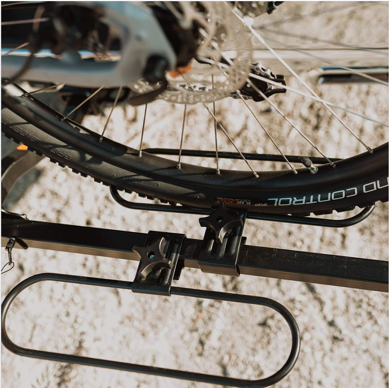
Image: Close-up view of the wheel hoops being installed onto the rack arms, showing the adjustment knobs.
