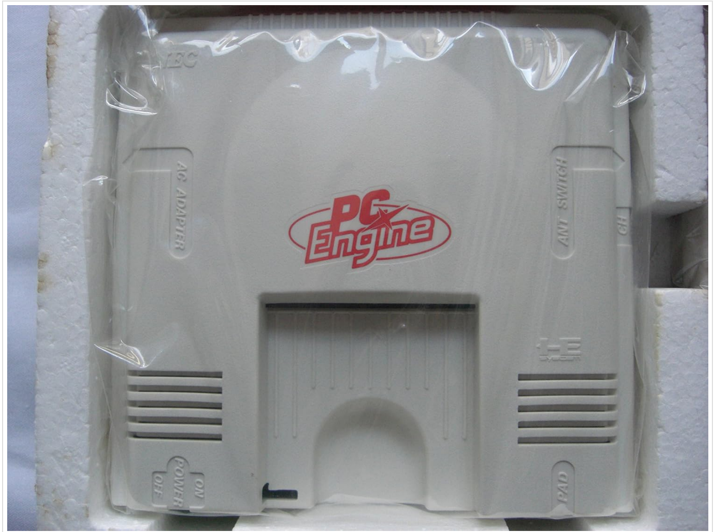
Image: A detailed top-down view of the NEC PC Engine console, highlighting the HuCard slot, power switch, and ventilation grilles, which are important for maintenance.
